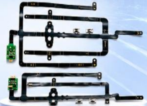
Double-Sided FPC + Surface Mount Technology
